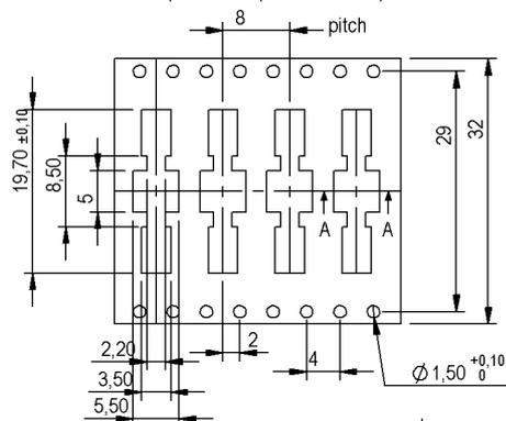
all dimension in this view are internal and are taken at the bottom of pocket draft angle is 20° except in center area where draft is 3°
