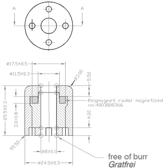
unspecified tolerance acc. to DIN/ISO 2768-m
