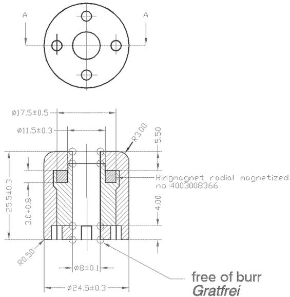
unspecified tolerances acc. to DIN/ISO 2768-m
